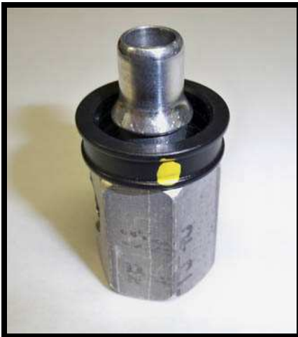
Figure 2 & 3. On the left the factory ring retainer is re-installed on the CNC male fitting. On the right a zip tie is used to retain the ring. Using a zip tie instead of the factory ring retainer is sometimes a better option as it is easier to remove later.
