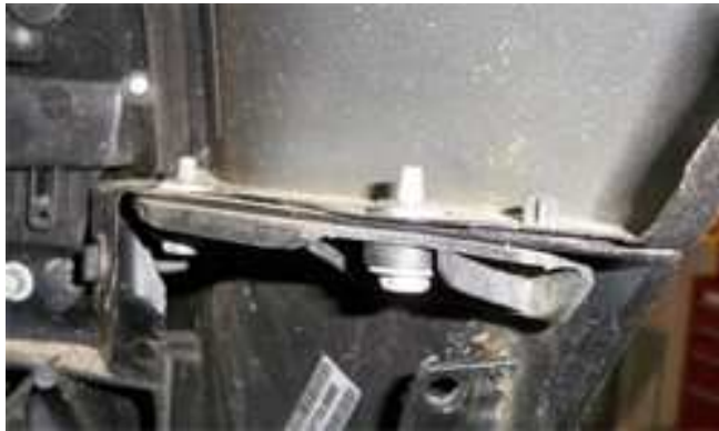
10mm bolts & recessed nuts holding bumper to fender
