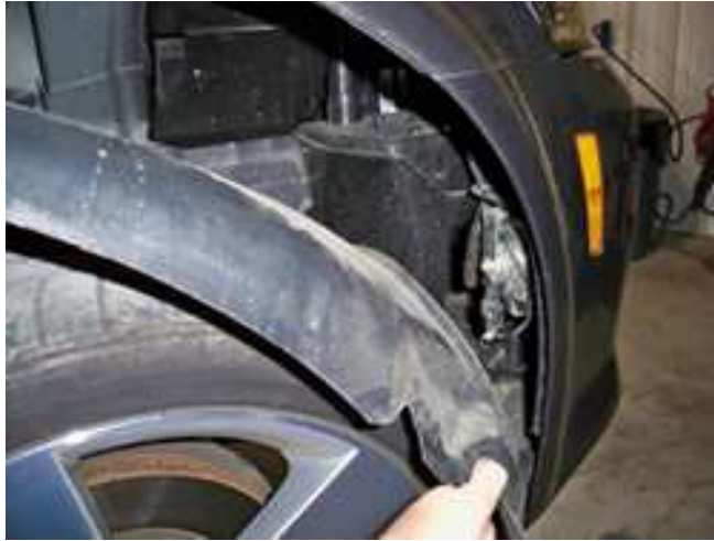
wheel well liner pulled out of the way
