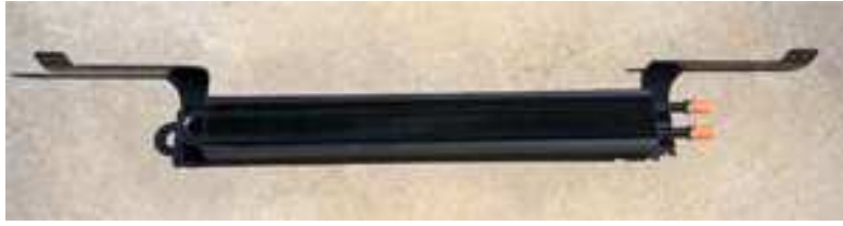
brackets attached to cooler
