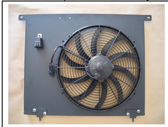
Figure 1 Fan and relay mounted to shroud
