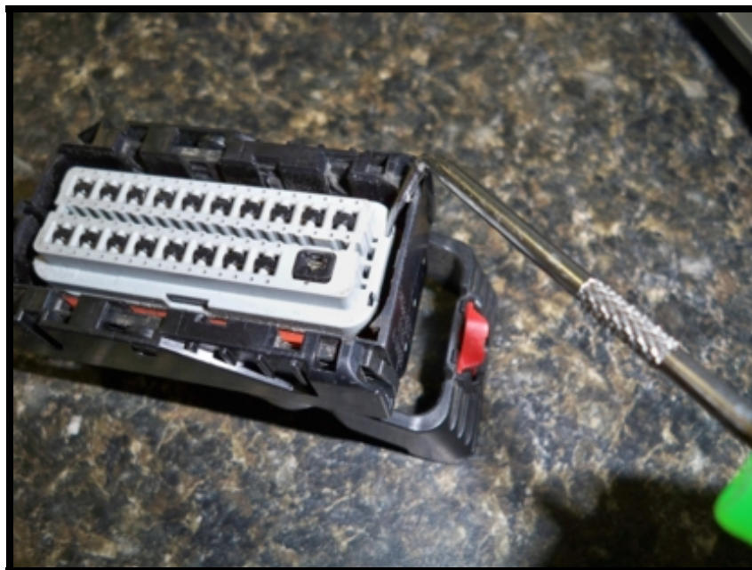
Figure 3 Remove connector face by pulling up from shown
