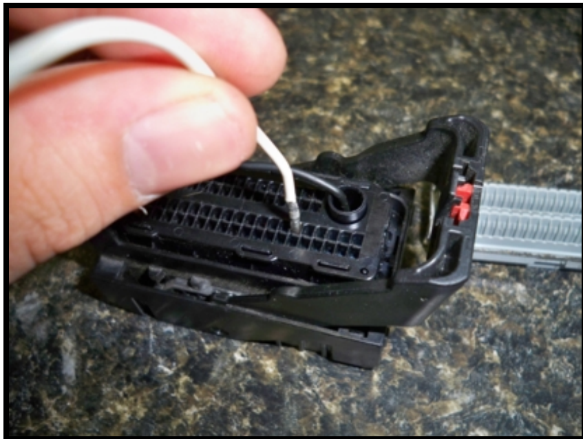
Figure 5 Inserting new pin. Will only go in one way
