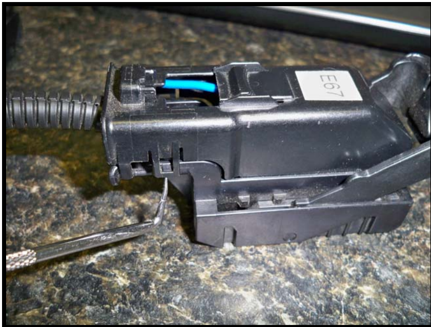
Figure 1 Release lock tabs for connector hood
