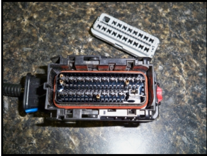
Figure 4 Connector face removed
