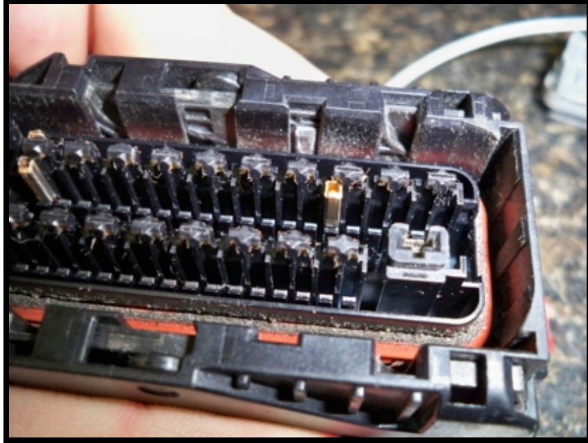
Figure 6 Pin seated fully
