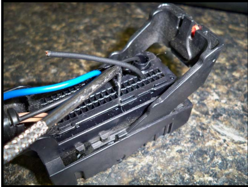
Figure 2 Clearing new pin hole
